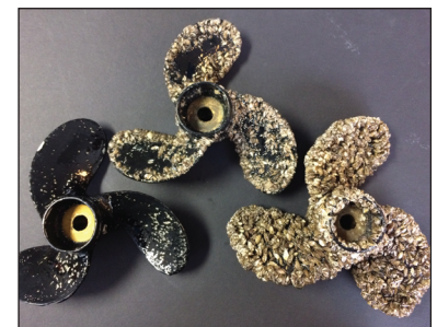
Adult zebra mussels colonizing propellers after 1, 3 and 4.5 months in an invaded water body.
