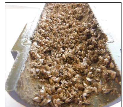
A cross-section of a pipe showing colonization of adult zebra mussels.
